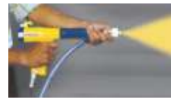
Cap at fully inserted position gives broader beam
