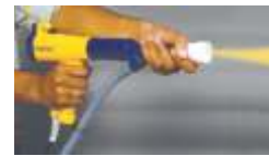
Cap at extreme position gives smaller beam
